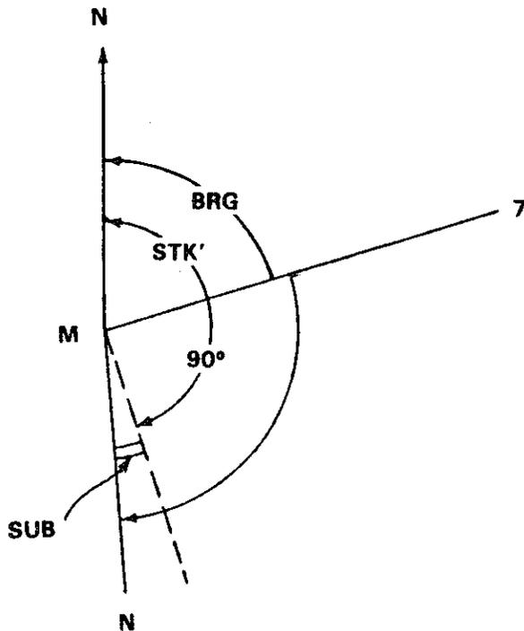
Fig. 4 Azimuth bearing angle, BRG, of line of intersection, M-N
