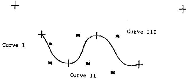
Fig. 3 Additional control points for the locally controlled Bezier curve
