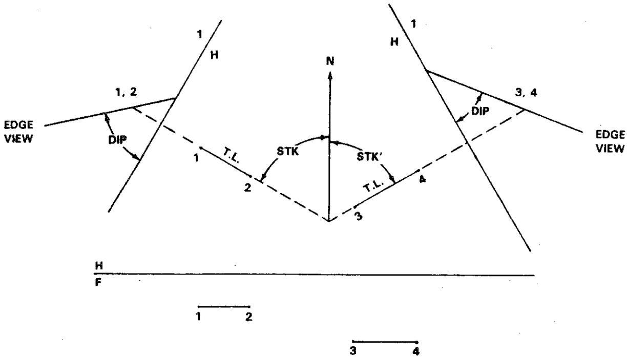
Fig. 1 Construction of edge views of given planes for strike and dip angles
