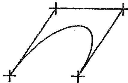
Fig. 1 Bezier curve and the characteristic polygon
