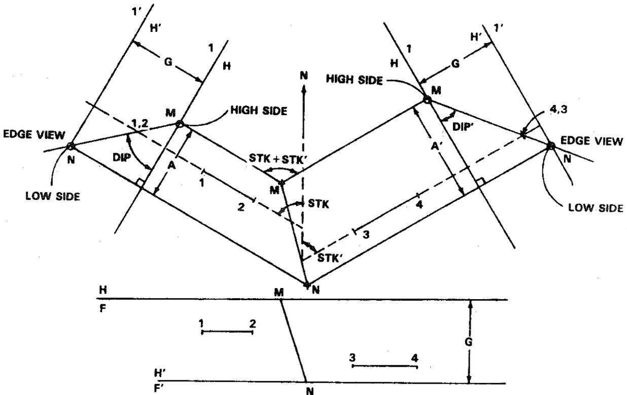
Fig. 2 Graphical solution to find line of intersection by auxiliary projection method
