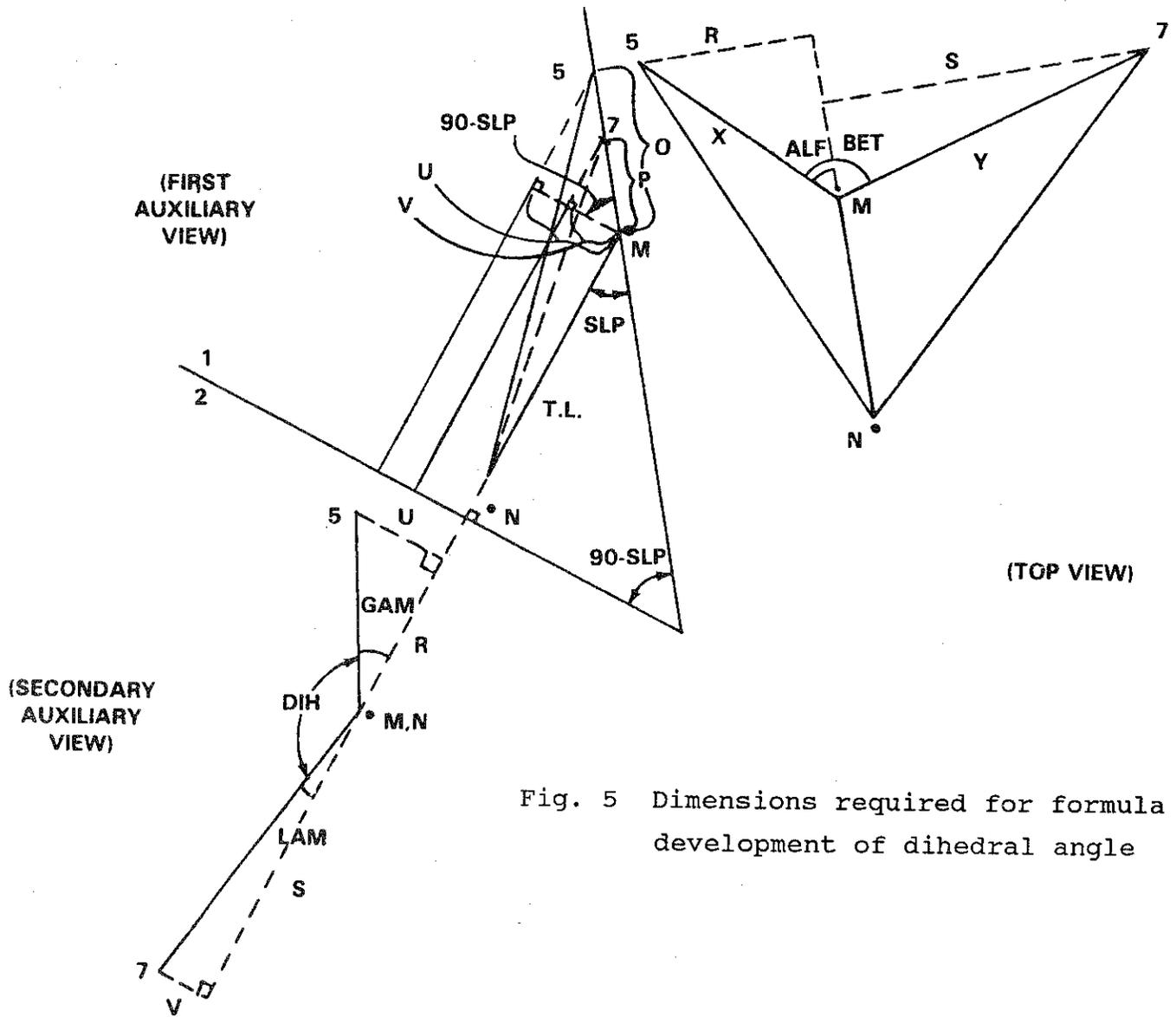
Fig. 5 Dimensions required for formula development of dihedral angle
