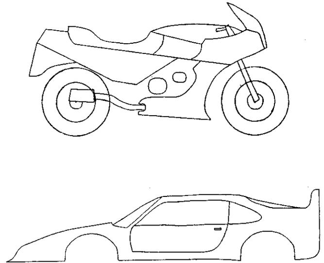
Fig. 7 Sample designs using multiple cubic Bezier curves
