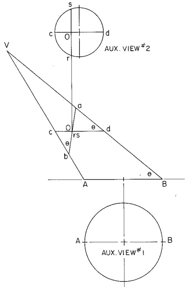
Figure 8: The determination of the angle between a line and a plane.
