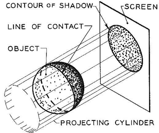
Figure 2: A collimated beam of light projects the contour of the object onto a screen.
