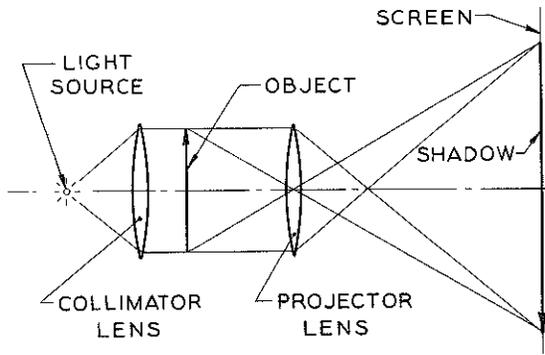
Figure 1: The optical system for projecting the object onto a screen.
