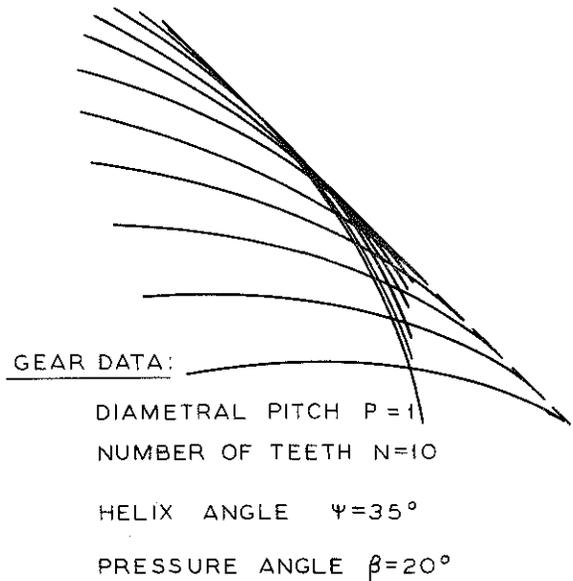
Figure 6: An example of a "HELGEAR" drawing to test the accuracy and profile of an involute helical gear tooth.
