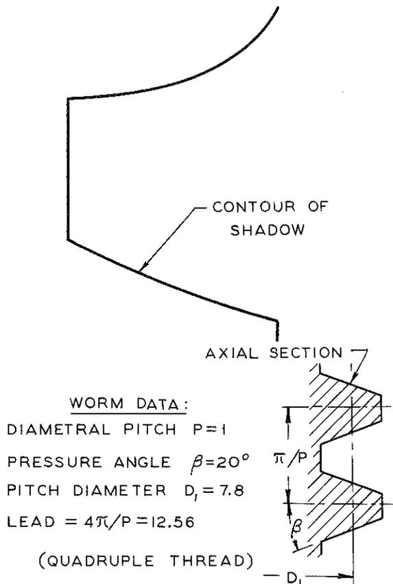
Figure 5: An example of a master drawing generated by "HEL".
