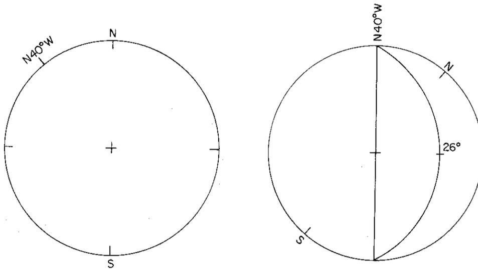
Figure 4: The construction of a plane having a strike of N 40° W and a dip of 26° NE.
