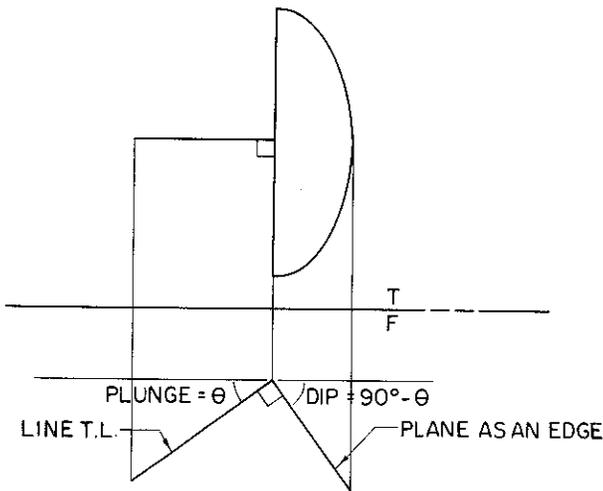
Figure 7: The determination of the angle between two planes.
