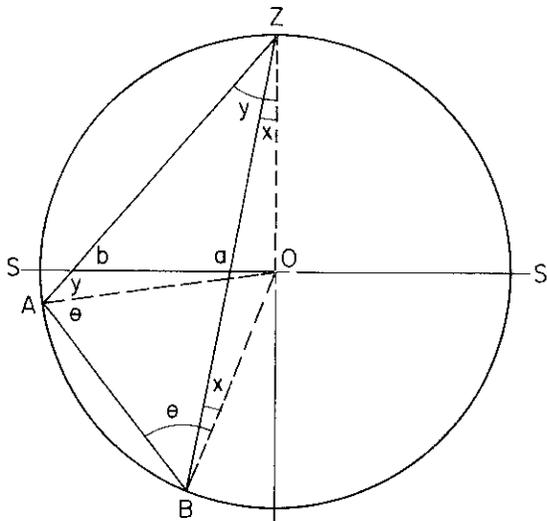
Figure 9: The circle is the orthographic projection of a sphere and AB is a circular section of the sphere appearing as an edge.
