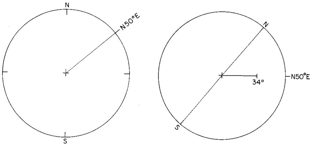
Figure 3: The construction of a line bearing N 50° E using a stereographic net.
