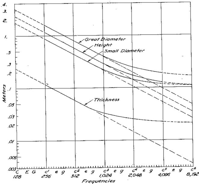
Fig. 3. The curves of proportion of the same series of bells, reduced to straight lines.
