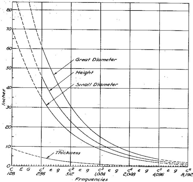
Fig. 2. The curves of proportion of a series of bells ranging from  $c^1$  to  $c^5$ .
