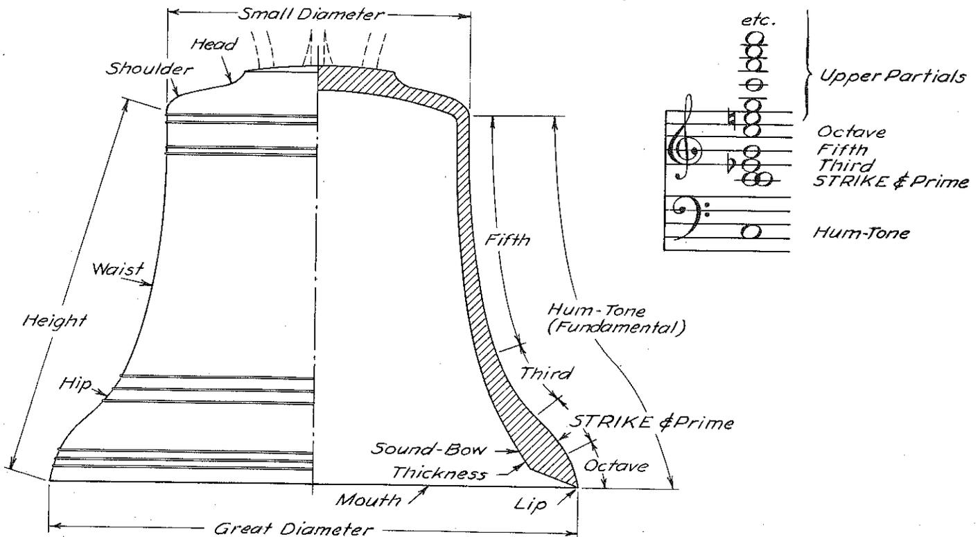
Fig. 1. The parts of a bell and its partials.
