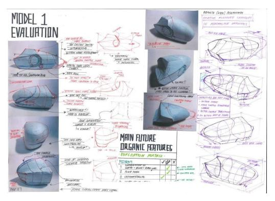
Figure 2. Example of student's iteration between sketches and foam model.
