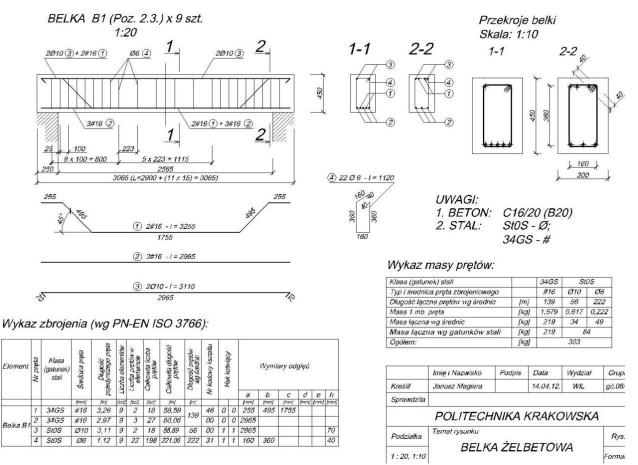
Figure 2. Example of a reinforced concrete structure: Beam and Bill of materials
