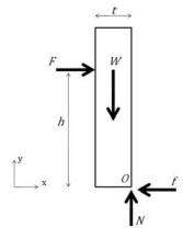
Figure 16. Free Body Diagram of a Domino
