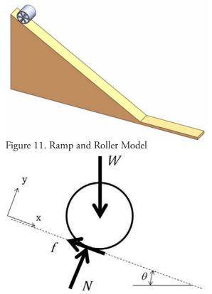
Figure 12. Free Body Diagram of Roller
