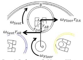
Figure 5. Configuration for Minimum Velocity
